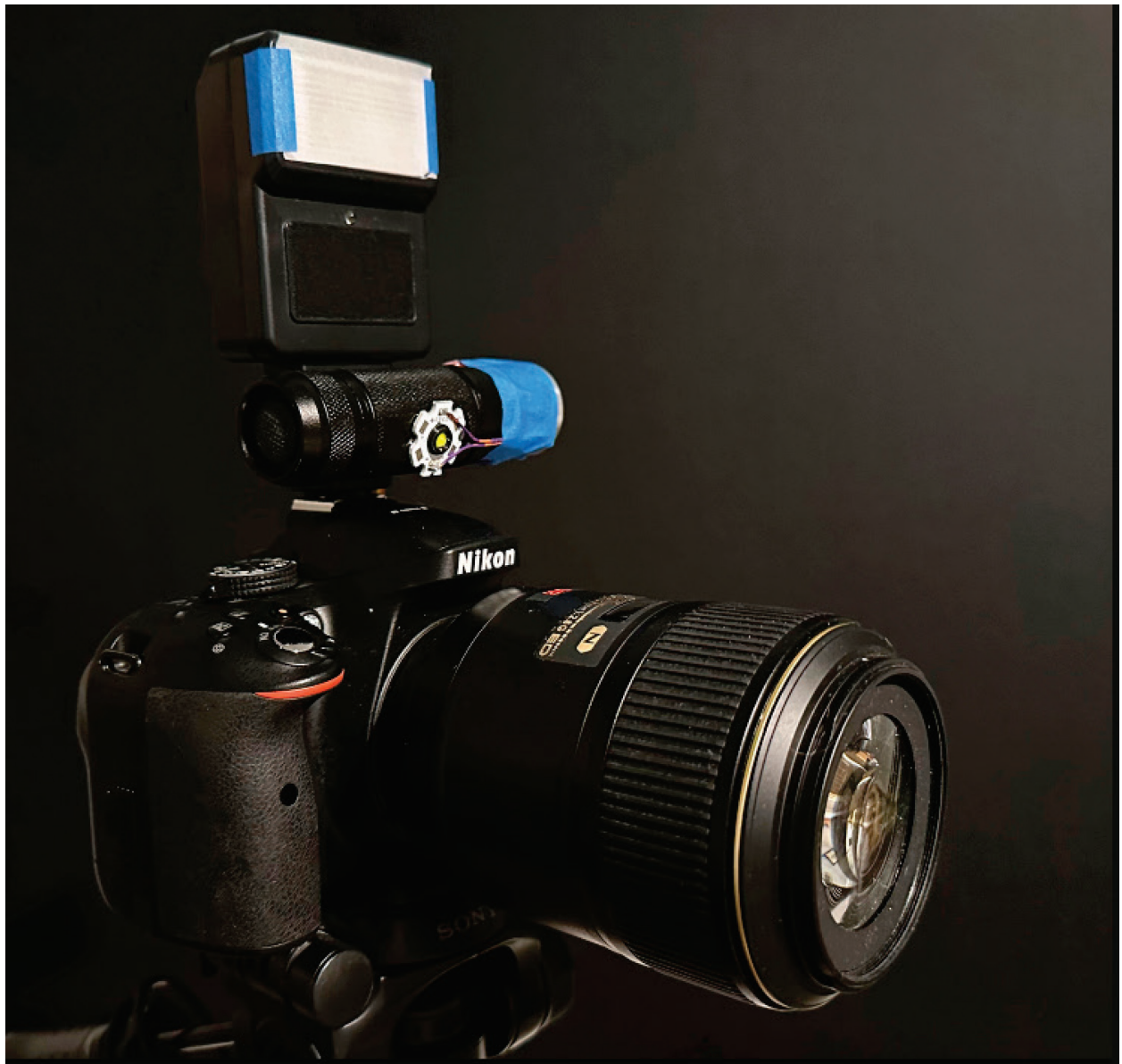
A hot shoe triggerable focusing light is ready for use.
